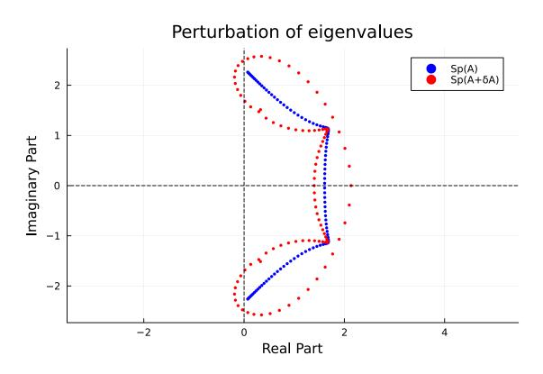
Hence, we see that, despite being well-conditioned for linear solves, the Grear matrix has illconditioned eigenvalues, which confirms that, indeed, the condition number is a problemdependent quantity.
